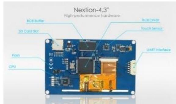
Gambar 9. Bagian-bagian Nextion NX4827T043\_011R [3].
